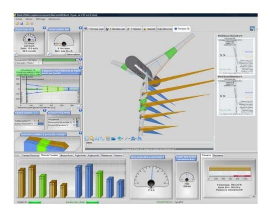
Another method of construction is possible to make an estimate of the performance of an existing propeller raising his pitch to different radius. This method of retro design is detailed on page "Performance and modeling of an existing propeller"
